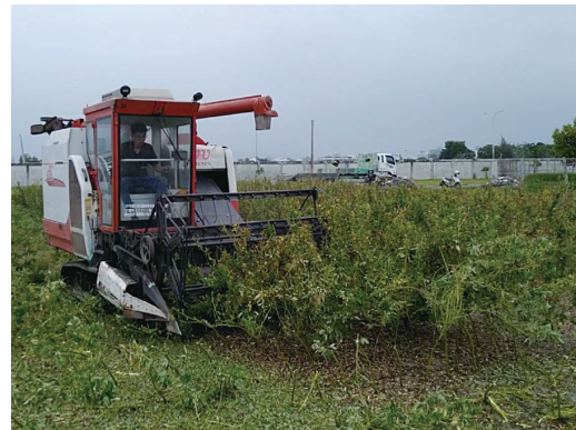
圖4. 雜糧聯合收穫機可將密植栽培樹豆莖部切斷（左）並採收（右） Fig. 4. The combine harvester can cut off and harvest the dense planting cultivation method of pigeon.
